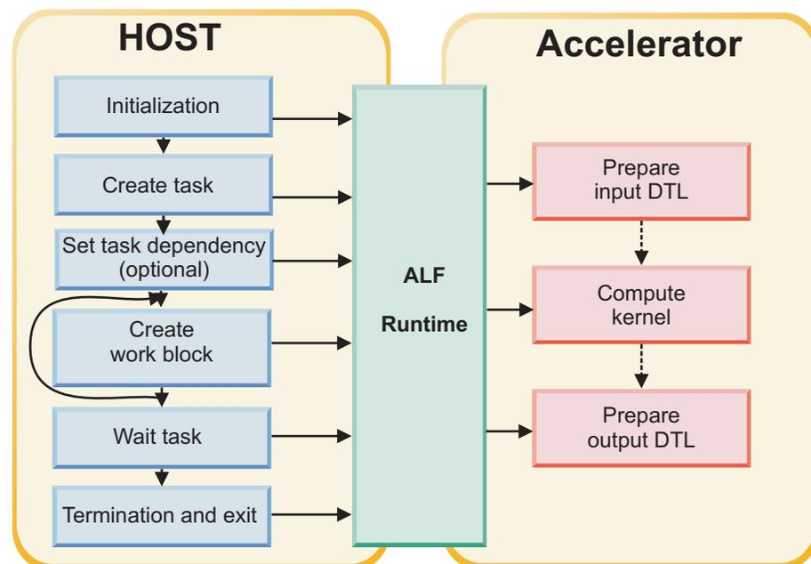
Figure 7. ALF application structure and process flow
